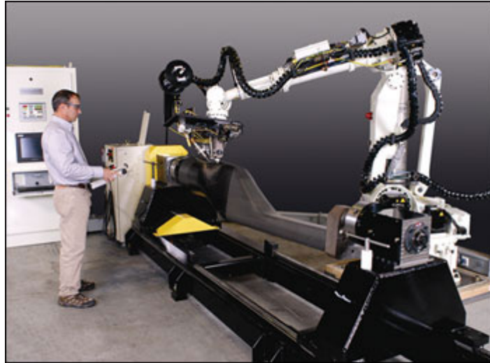
Automated Dynamics is looking to robots for affordable automation. The company recently announced its AFP/ATL-0510 robot system for tape laying or fiber placement.
