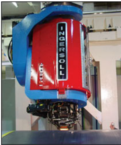
The Mongoose V1 recently completed qualification tests, laying thermoset composite at 60 lb/hr (27 kg/hr) over a test fuselage section. An articulated head allows it to operate inside molds as well as outside mandrels.
