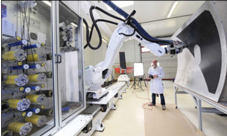
The Coriolis robotic system lays thermoset, thermoplastic, or dry fiber, and is capable of concave as well as convex deposition.
