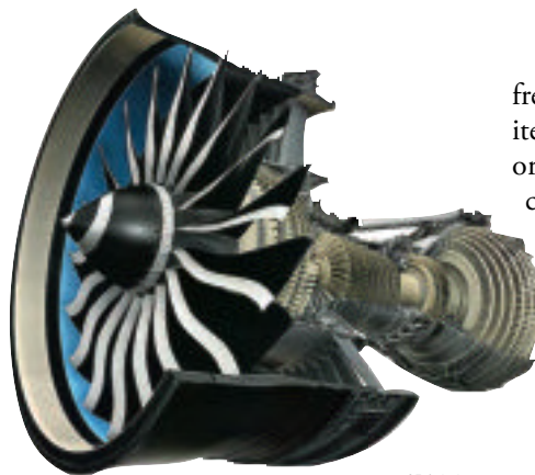
GE Aviation The GENx is GE's next-generation turbofan engine for medium-capacity, long-range aircraft, including the Boeing 787 Dreamliner.
