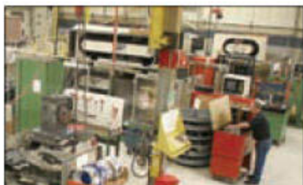
The four 4- and 5-axis Mitsui Seiki horizontal CNC machining centers are staged with custom modular fixtures to ensure exceptionally fast setups and secure workholding for gearbox manufacturing precision (courtesy Triumph Gear-Macomb).
