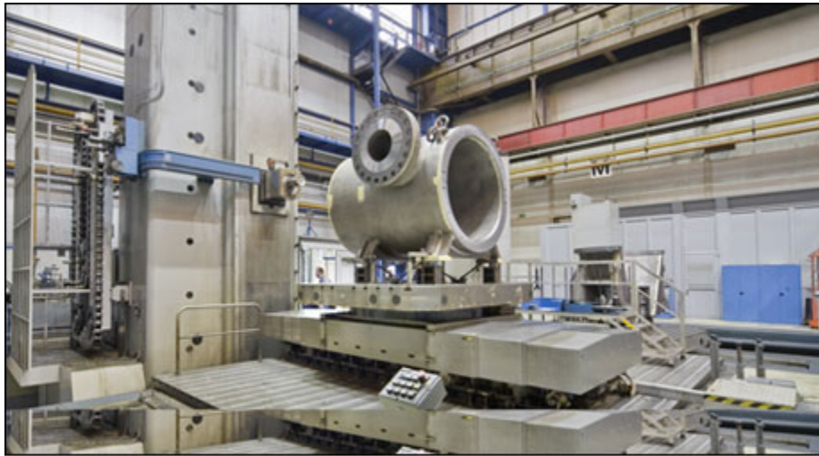
Massive size of parts for energy industry can be seen on a boring and milling machine with 100-t rototraversing table and 100-kW spindle at Siemens AG's Duisburg Energy division plant. Photo courtesy PAMA Inc.
