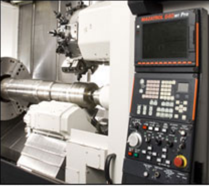
Mazak Cybertech Turn 5500's turret design allows easy visual realignment for rethreading.
