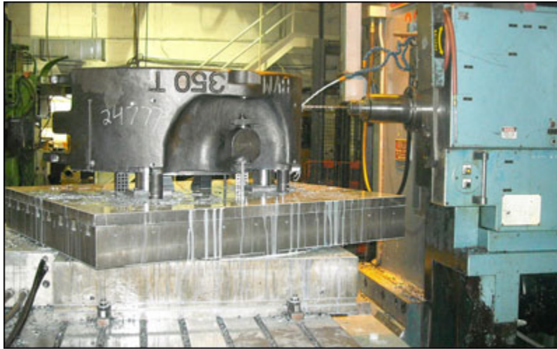
Deep-hole drilling in large energy-industry components requires tooling strategies to match the available technology. Photo courtesy OSG Tap & Die
