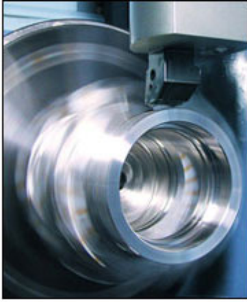
Complex parts can be turned and milled on the Cublex 25PC 400. Photo courtesy Methods Machine
